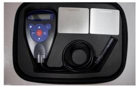
This device is a portable meter. It is capable of measuring coating thickness quickly, precisely and without injury, both for the laboratory and engineering environment. It is currently widely used in manufacturing, metal processing industry, chemical industry, commodity inspection and testing fields, and is essential for material protection major.
